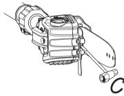
The chain is correctly tensioned when there is no slack on the underside of the bar, and it can still be turned easily by hand. Tighten the bar nut with the combination spanner while holding up the tip of the bar.
